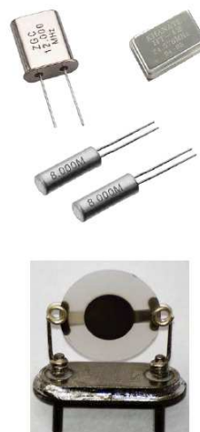
Fig. 4- 13 Crystal enclosures and mounting
