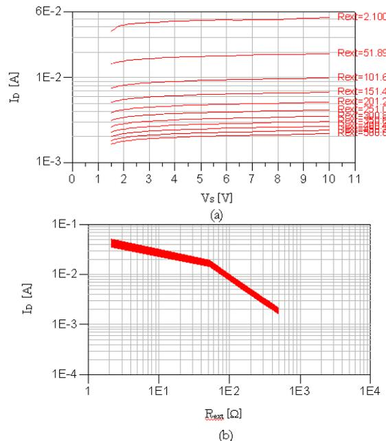
Figure 3. Characteristic curves of BCR400W (a)  $I_D$  vs  $V_D$  and (b)  $I_D$  vs  $R_{ext}$
