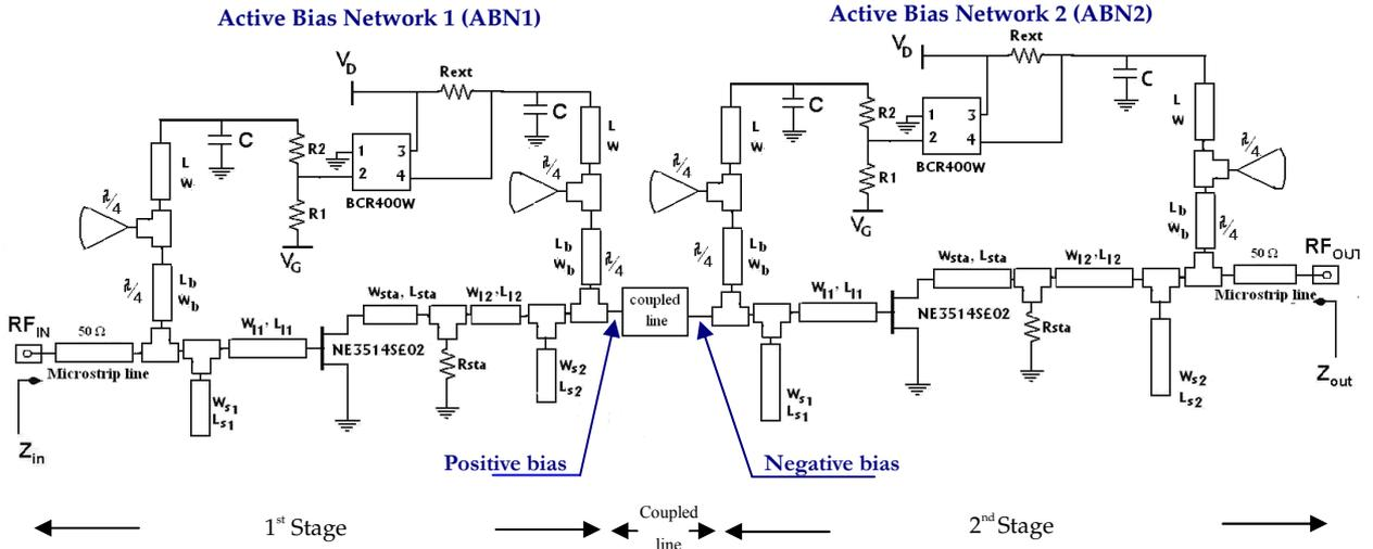
Figure 8. Electrical schematic of two-stages 24 GHz LNA based on NE3514S02
