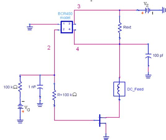
Figure 2. Electrical schematic of biasing of the transistor by a BCR400W
