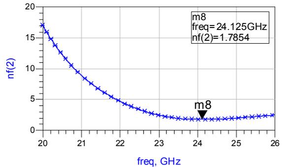
**Figure 5.** Noise Figure vs. Frequency
