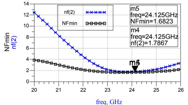
Figure 10. Noise Figure vs. Frequency
