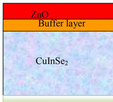
Figure 1: ZnO window layer/Buffer layer (CdS or ZnS or i-ZnO)
