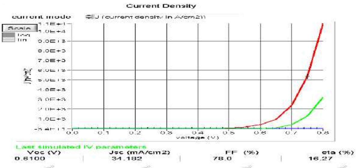
Figure 1: I(V) curve for ZnO window/ CdS buffer/ CIS solar cell
